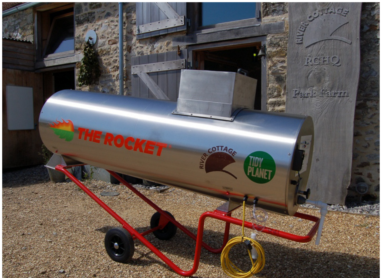
The A500 Rocket in vessel composter, providing “closed loop” on site food waste recycling at the River Cottage in Axminster.
